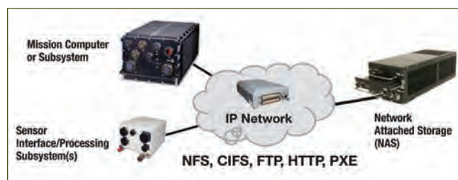
Figure 1 | The NAS/file server is designed to provide file services to clients on an IP network.
